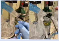
Turn off the heater by holding down on the power button (bottom right button) for around 1-2 sec.
